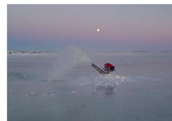
Flooding pump with submersible auger. (Masterson, 2009)
