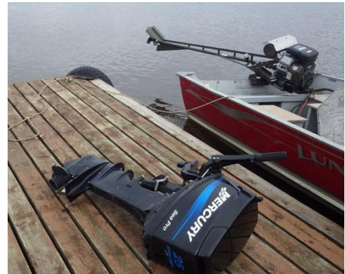
Common outboard motors can be damaged when used in shallow water. Mud motors or jet motors may be better options.
