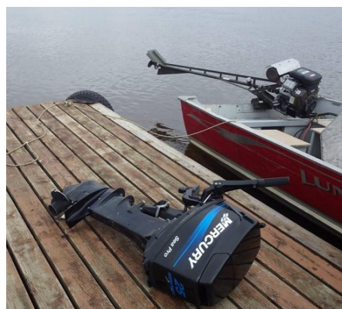
Common outboard motor is replaced by a mud motor to navigate better in shallow water and reduce damage.
