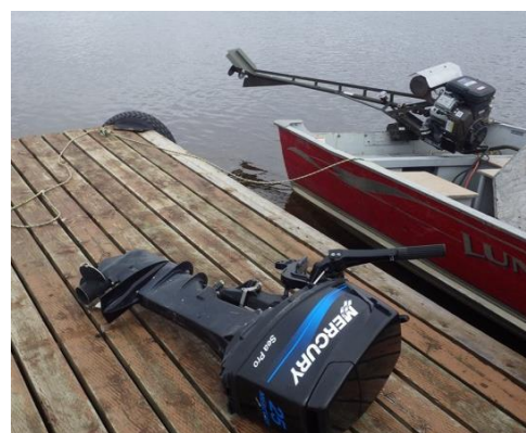
Common outboard motors can be damaged when used in shallow water. Mud motors or jet motors may be better options.
